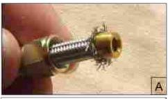
Push the olive onto the end of PTFE inner tube and under the stainless steel braid. Make sure that all stainless steel filaments are outside of the olive.
