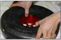
**BE CAREFUL this operation is delicate !** Pull up the tire and push the wheel at the same time with the thumbs.
