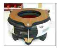
Place the second part of the special tool then insert the 3 bolts. Press the tire with the tool till the tire flange is totally under the level of the horizontal surface of the wheel. Clean the horizontal
