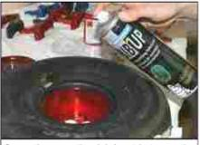
Spray tire mounting lubricant between the tire and the wheel.
