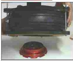
Place the whole assembly on the wheel flange as shown above BE CAREFUL: The O-ring must stay in the ring groove during this operation.
