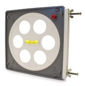
You should be pleased to know that you are using the Warp Drive Professional Protractor which is designed after the high dollar propeller protractors. When used properly this protractor used on Warp Drive propellers, aircraft propellers or airboat propellers, can help you set your propeller blades pitch angle within 1/4 of a degree. It can also be used to check wing surfaces on your aircraft.
