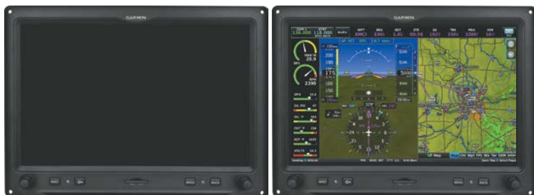
G3X Touch Full-Screen Reversionary Mode (Failed PFD)
