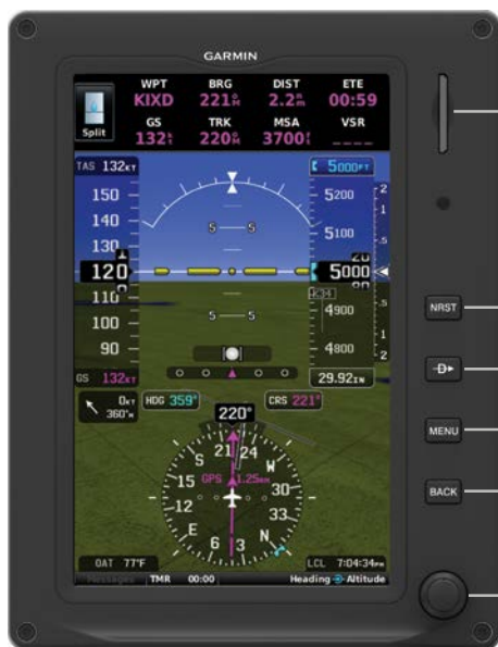
Left Knob Nearest Button Direct-to Button SD Card Slot Menu Button Back Button Right Knob
