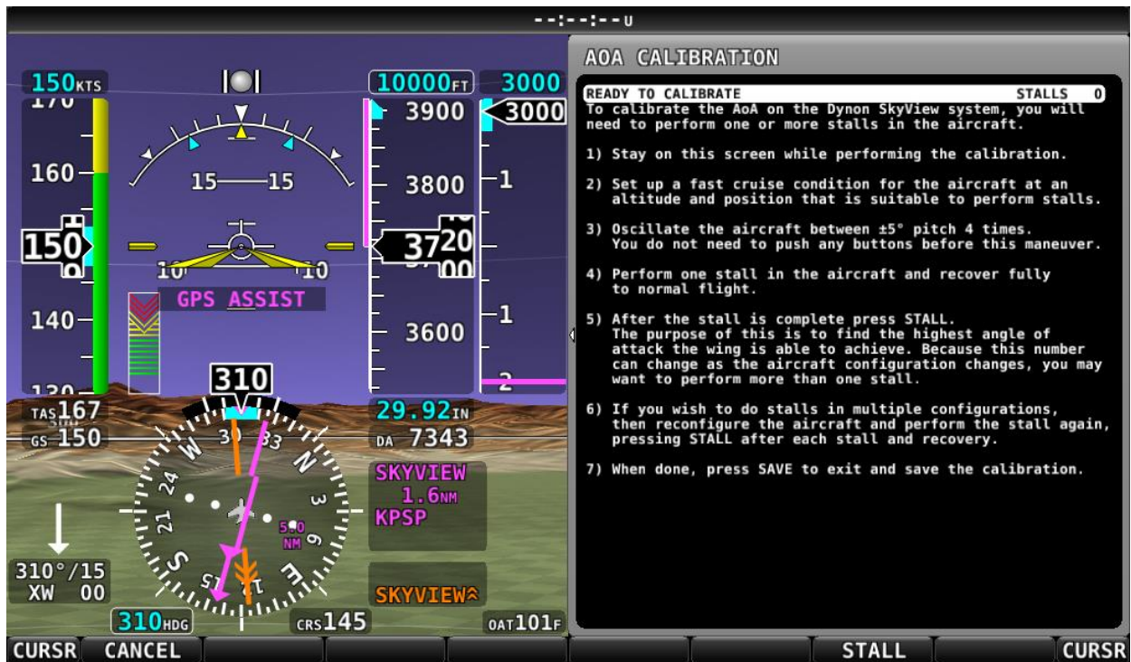
Figure 169 – AOA Calibration Explanation and Wizard
