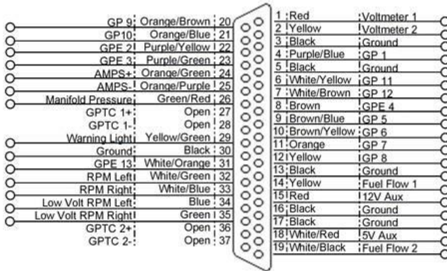
Figure 59 – SV-EMS-220 37-pin Main Sensor Harness D37F Pin Insertion View (Rear)
