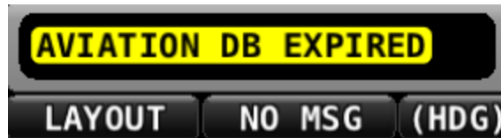
Figure 52 – SkyView SE Aviation Database Expired Caution Message (Lower Left Corner of Display)
