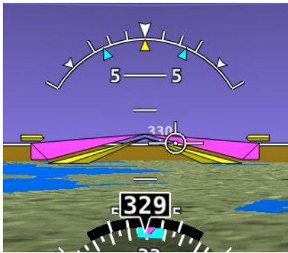
Figure 122 – Flight Director - Single Cue (Inverted-V)
