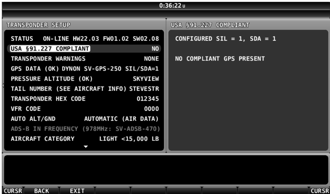
Figure 143 - 14 CFR § 91.227 Compliance Status – Not Compliant
