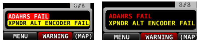
Figure 237 – Unacknowledged (left) and Acknowledged (right) Alarms
