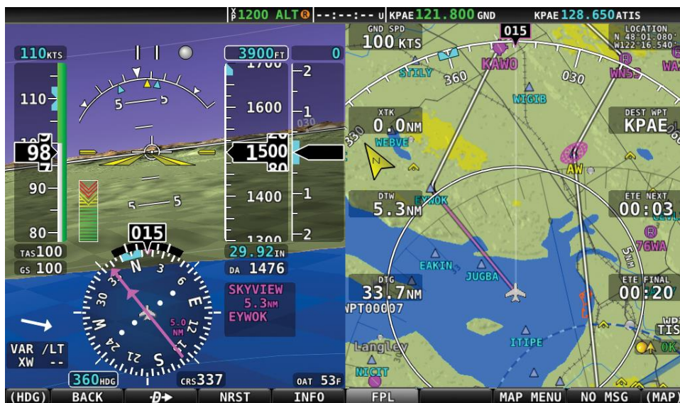
Figure 148 – Active Flight Plan: HSI and MAP Depictions
