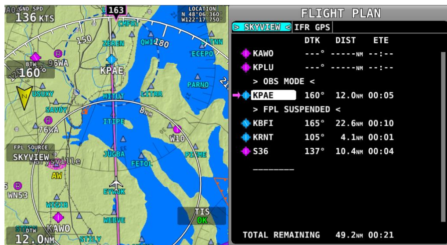
Figure 149 – OBS Mode Activated
