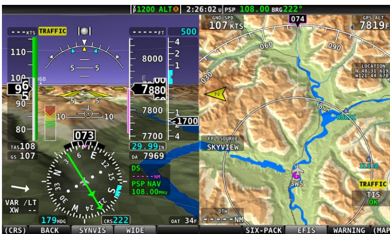
Figure 45 – SkyView Synthetic Vision Wide View
