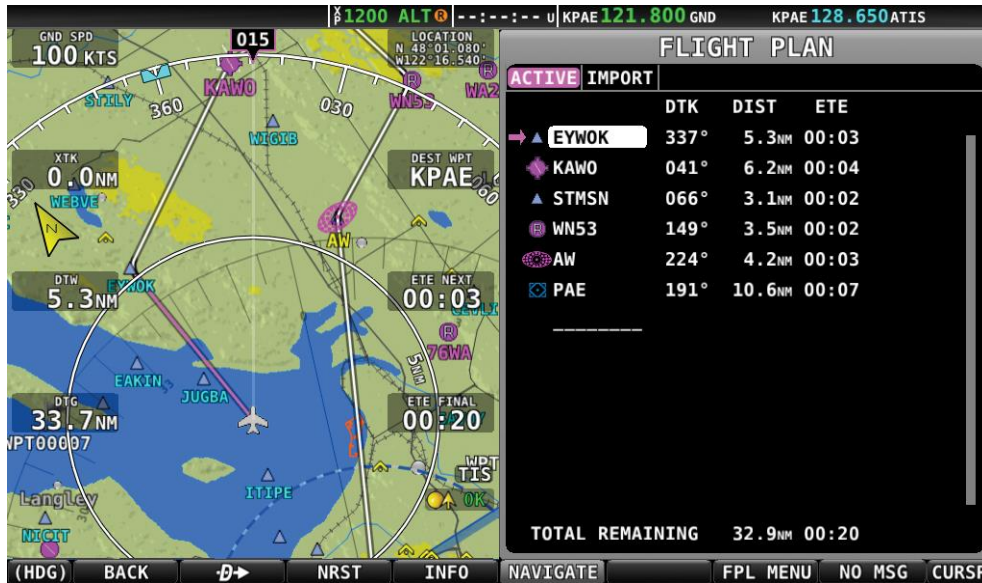
Figure 147 – Active Flight Plan: Map and Flight Plan View
