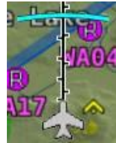
Figure 84 – Altitude Intercept Arc
