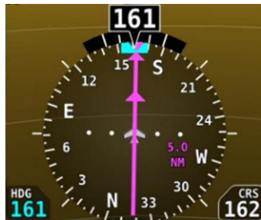
Figure 26 – HSI Example - Localizer
