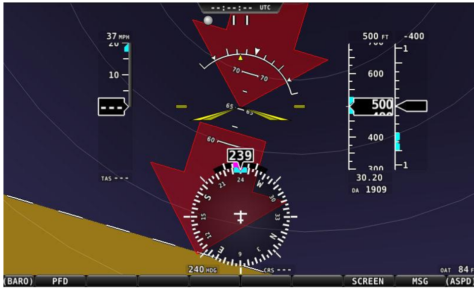
Figure 52 – Extreme Pitch Warning Indicator Arrows
