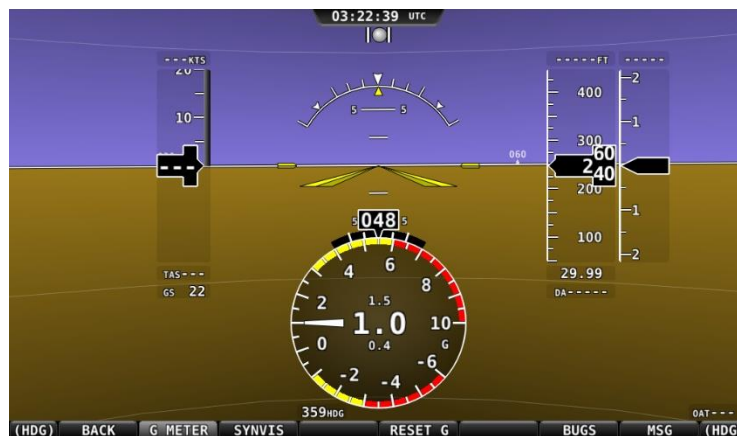
Figure 60 – G Meter on PFD
