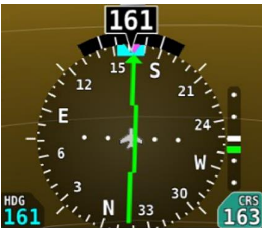
Figure 25 – HSI Example: GPS
